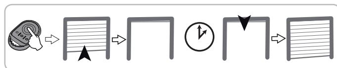
A new command during this time delay cancels automatic closing and the door remains open.
